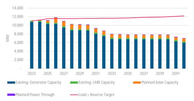
Figure 10: ELL Capacity Position
