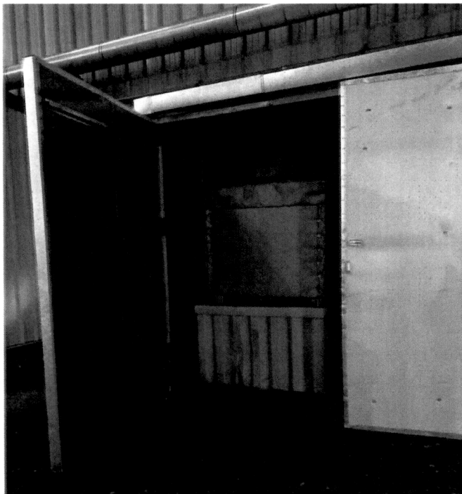
Figure 11: Heated Blankets on Cones Downspout of Silos
